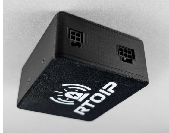
Power side with logo upright: BAT 4-pin (left) and FLASH 6-pin (right).
